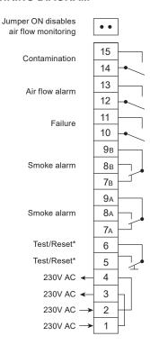
The relay outputs are shown in power off/alarm condition.
